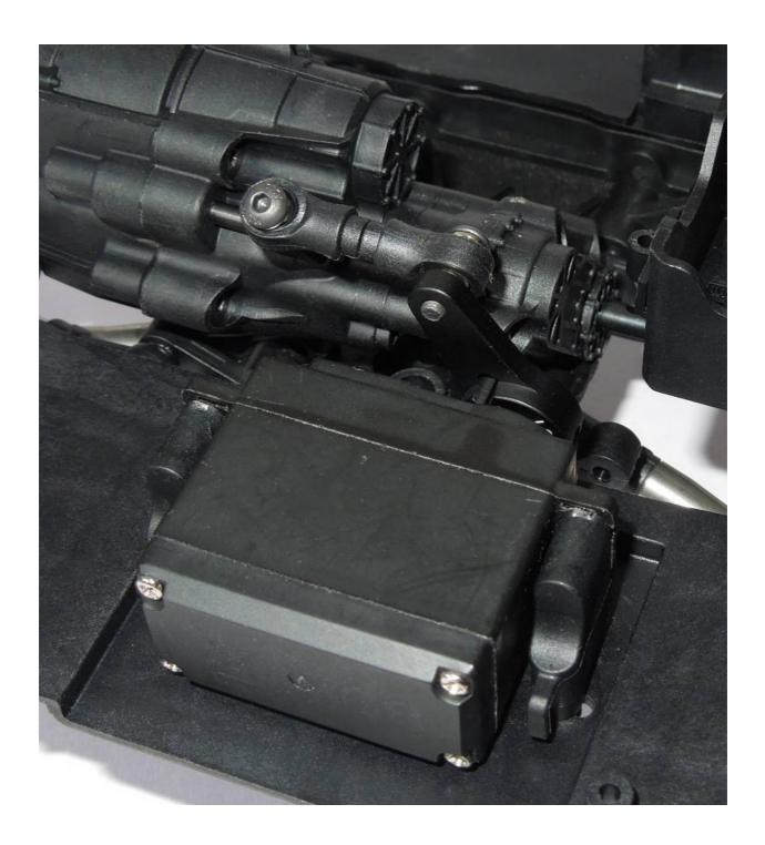
**Note:** A 3 channel radio is needed in order to connect the shift servo and change gears.
